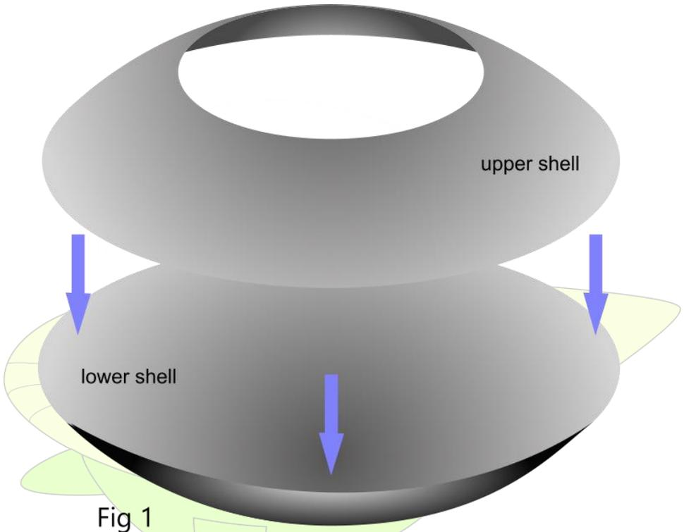
Whilst it will benefit from internal stiffening, this will be very simple to incorporate and comprises multiple internal ribs of exactly the same shape, size and strength. The ellipsoid shape minimises drag-resistance when travelling horizontally through an atmosphere.
