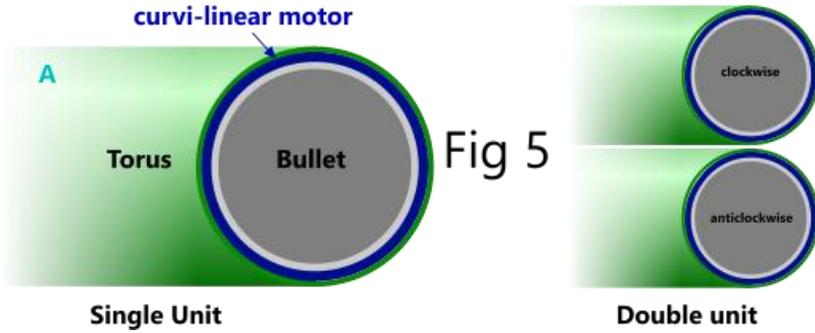
Both of these problems may be avoided by careful reconfiguration such as described in Appendix A3; Fig G. In all such configurations, it is important to balance Bullet-mass to eliminate system torque (and vibration).
